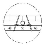
(6) Insert connection bar into SPTM-6VL feedback lever. The connection bar should be inserted at the 50% point on the feedback lever, which would help to reduce hysteresis. <Fig 4>
